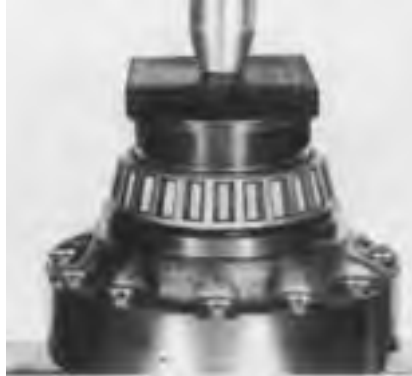
2. Press bearing cone on plain differential case.
