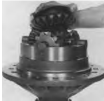
5. Place side gear and thrust washer on side pinions.
