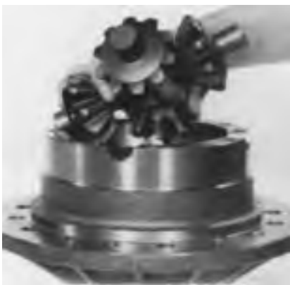
4. Assemble side pinion and thrust washers on spider. Place this assembly in flanged differential case. Rotate gears and check for proper mesh.
