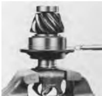
Measuring Bearing Preload with Pinion in Vise.
