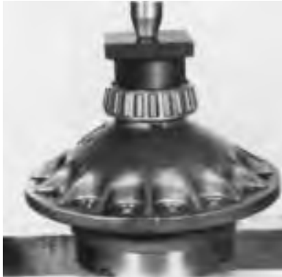
1. Press bearing cone on flanged differential case.
