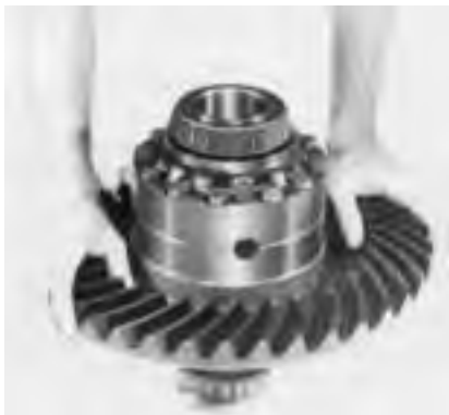
7. Install ring gear. Secure with bolts and nuts and tighten to correct torque (see chart).
