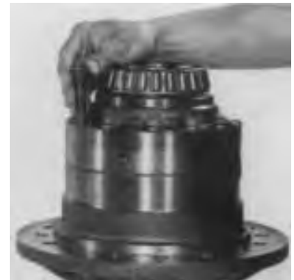
6. Align punch marks and install plain case half. Install cap screws and tighten to correct torque (see chart).
