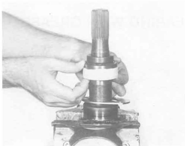
Figure 40 1022-40 Pull the seal towards the bearing until it contacts the rib ring. This will force the grease between the rollers and the cup.
