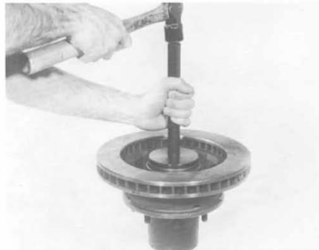
Figure 12 1022-12 Assemble new grease seal. Apply a small amount of grease around lip of seal. Tools: D-253 Seal Installer, C-4171 Handle.
