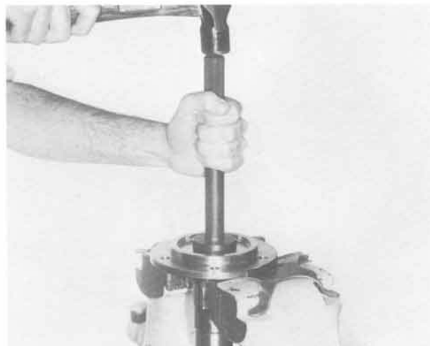
Figure 42 1022-42 Assemble new needle bearing into spindle. Tools: D-258 Installer, C-4171 Handle.
