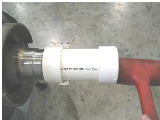
Install sleeve with Driver
