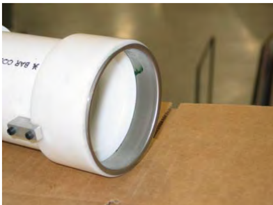
Rolled Lip Should Face Outward
