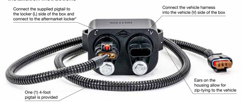
\*Connect directly to an electric locker or connect to the air solenoid for air-locking differentials
