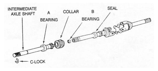
When replacing the Intermediate Axle Shaft, the needle bearing "B" should be replaced with synthetic bushing, 43337, contained in the above-mentioned kit, 75265X.
