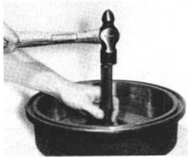
Figure 12 1010-12 Remove inner and outer wheel bearing cups. Tools: #D-256 Cup Remover, #C-4171 Handle.
