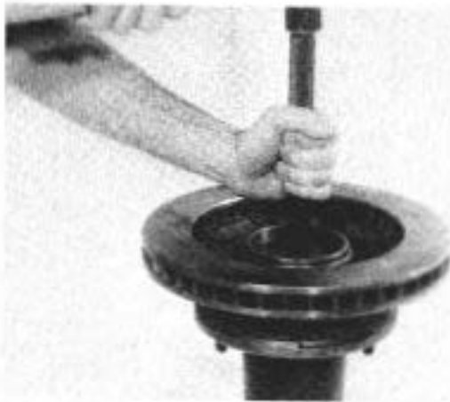
Figure 50 Assemble inner wheel bearing cup. Tools: #D-254 Installer, #C-4171 Handle.
