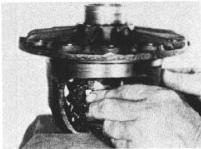
Figure 158 Place differential case in view as shown. Apply grease to new side gear thrust washers and to hubs and thrust face of the new side gears. Assemble both side gears. Apply grease to the new cylindrical washers, and the new pinion mate gears. Assemble new pinion mate gears and washers.
