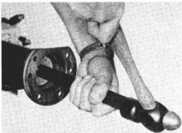
Figure 92 1018-02 Assemble new grease seal into housing. Tools: #C-4026A Seal Installer, #C-4171 Handle. After seal has been assembled, grease lip of seal.
