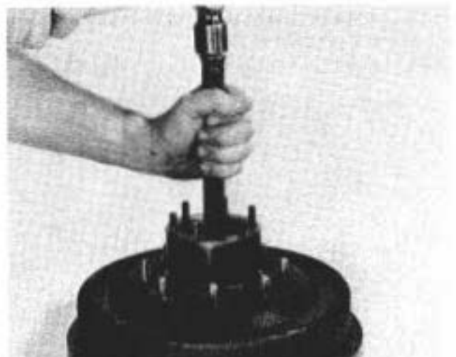
Figure 13 1010-13 Assemble outer wheel bearing cup. Tools: #C-4023 Installer, #C-4171 Handle.
