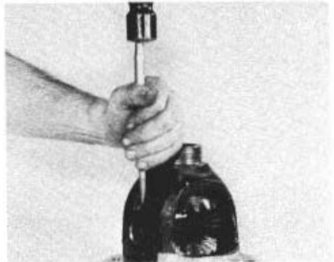
Figure 160 Assemble lock pin. Push metal of case over pin to lock in place.
