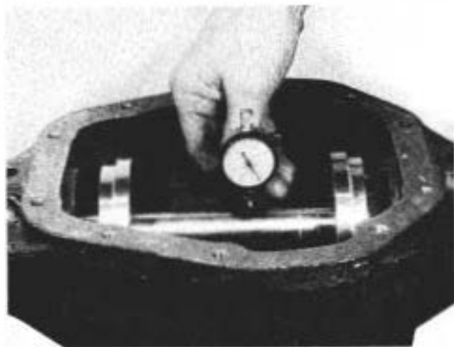
Figure 173 1012-173 Slide scooter gage over arbor. As gage slides over top of arbor, it will travel in a clockwise direction. When indicator is on center of arbor (top) it will stop traveling in a clockwise direction. If indicator starts to travel in a counter-clockwise direction, this means you have passed the center of the arbor. Record only the reading when the indicator is at the highest point. This reading indicates the amount of shim necessary to obtain the shim pack, plus (+) or minus (-) the etching on the bottom end of the pinion. If the etching is zero (0), the shim pack will remain unchanged. For example: If the pinion is etched +3 (m+8), this pinion would require .003" (.08 mm) less shims than a pinion etched zero (0). If the pinion is etched -3 (m-8), this would require .003" (.08 mm) more shims than a pinion etched zero (0).
