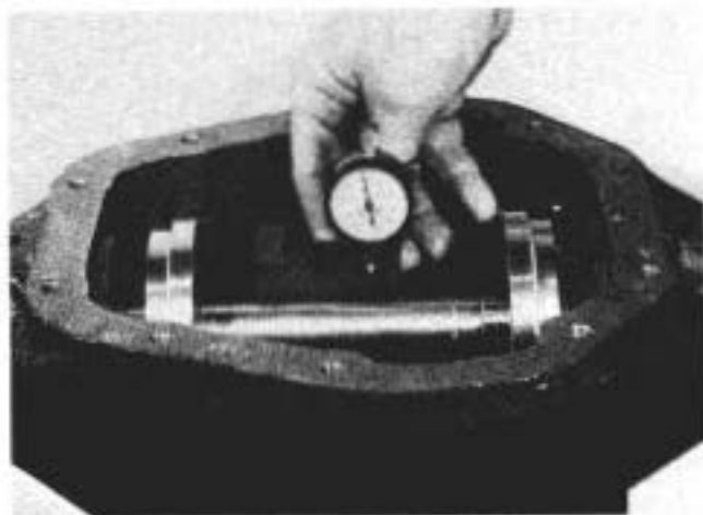
Figure 172 1012-172 Place scooter gage on small step of pinion height block. Apply pressure with fingers, making sure the gage is flat on the pinion block, while pressure is applied set indicator at zero "0". Tool: #D-116 Scooter Gage.
