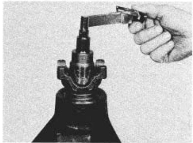
Figure 182 1010-182 Using an In. Lb. torque wrench as shown, rotate pinion. Torque to rotate pinion should read between 20-40 Lb. In. (2.26-4.53 N-m). To increase preload, remove shims; to decrease preload add shims.
