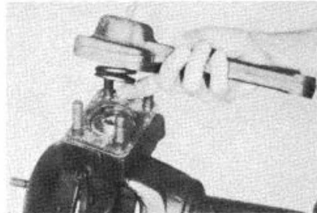
Figure 57 101B-57 Remove steering arm, compression spring, and gasket. Discard gasket, replace with new one at time of assembly.
