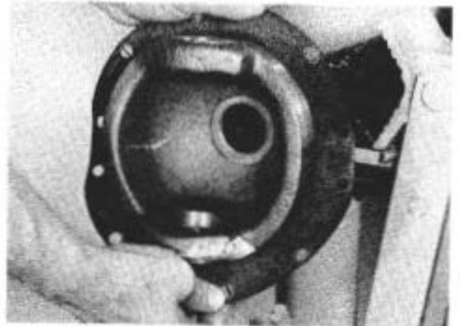
Figure 32 1019-32 Assemble new felt over spherical ball as shown.
