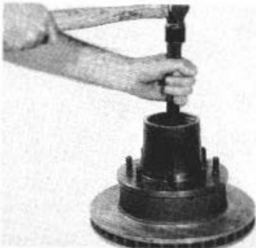
Figure 49 Assemble outer wheel bearing cup. Tools: #D-254 Installer, #C-4171 Handle.
