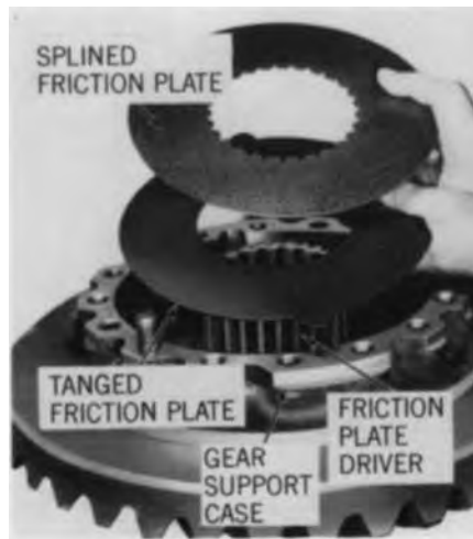
Installing Friction Plates
