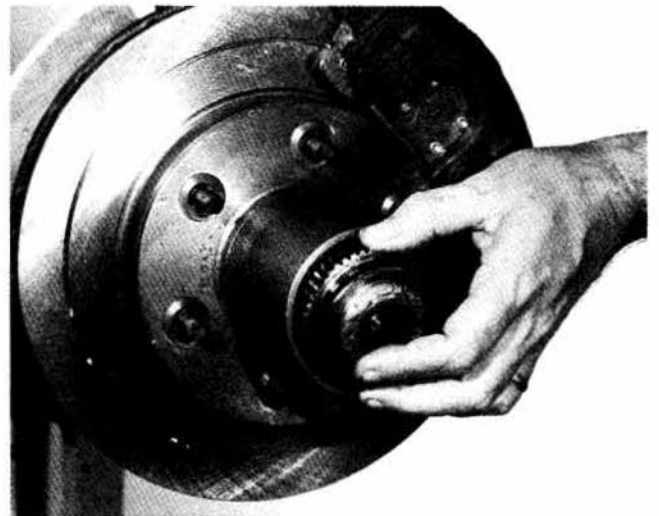
Figure 16 1005-14 Assemble inner clutch ring and axle shaft sleeve if face tooth design or outer clutch ring and inner clutch ring if sliding tooth design. Notice that the teeth are meshed together in a locked position for easy assembly. Refer to exploded view for proper parts orientation and identification. It may be necessary to rock the hub back and forth for spline alignment. Keep the two clutch rings in LOCKED position. Assemble axle shaft snap ring. Be sure snap ring is fully seated in the snap ring groove of the shaft.
