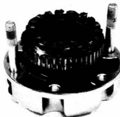
Figure 8 1001-18 Assemble two screws with washers into lockout hub housing. Apply a small amount of Moly XL hi-speed grease to the outer spline and teeth of the outer clutch gear. Remove any excess lubricant from the gasket surface of the retainer.
