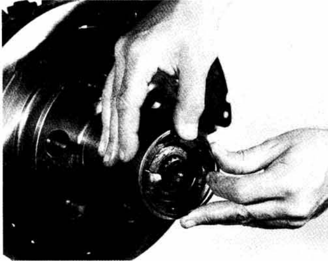
Figure 18 1005-17 Assemble hub snap ring. Be sure snap ring is fully seated in the snap ring groove of the hub.
