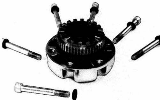
Figure 7 1001-17 Assemble six dished washers to the six retainer screws.
