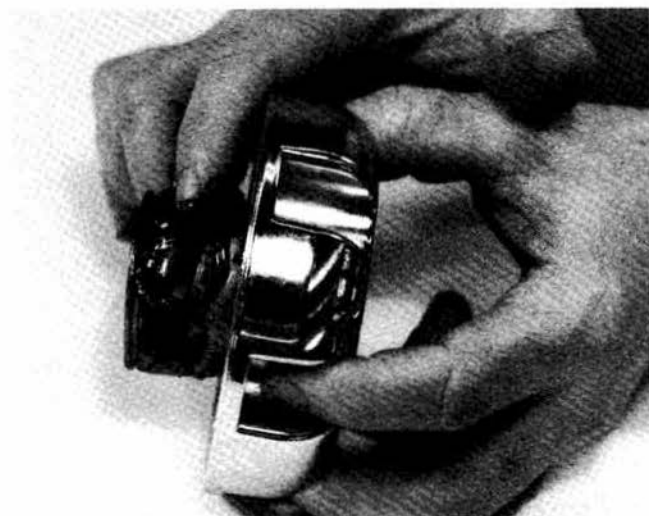
Figure 5 1001-15 Turn actuator knob to LOCK position. Apply a small amount of Moly XL hi-speed grease to both grooves of the cam as shown.
