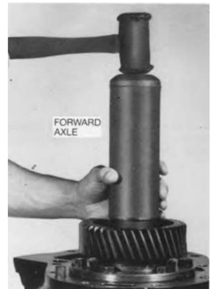
Installing Pinion Helical Gear.
