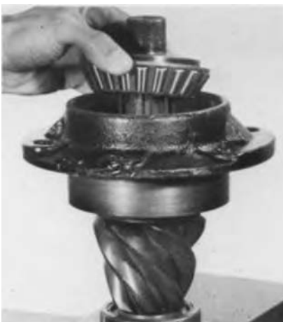
Removing "Slip-Fit" Outer Bearing Cone (Rear Axle illustrated).
