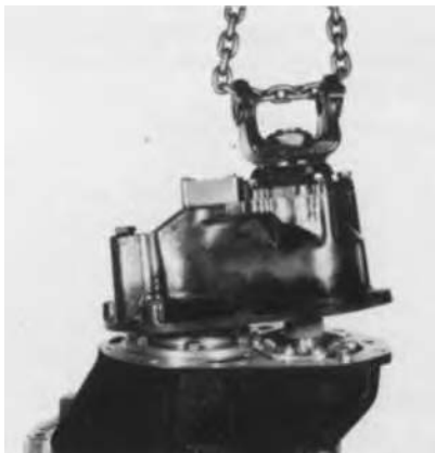
Power Divider Cover Dowel Pin Location.
