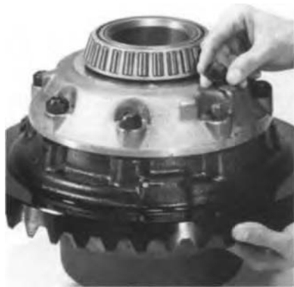
1. Remove nuts and bolts fastening ring gear and support cases.
