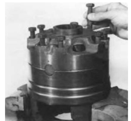
7. Punch mark differential cases for correct location in reassembly. Remove cap screws and separate case halves.
