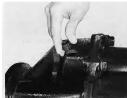
Oil Filler Hole at top of Differential Carrier.
