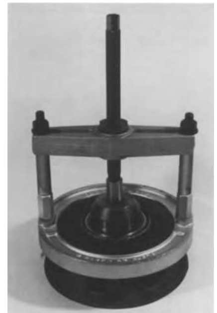
Removing Bearing from Small Support Case using Puller.
