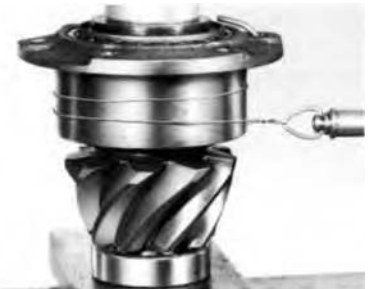
Measuring Bearing Preload with Pinion in Press.
