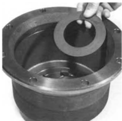
5. Remove thrust washer from support case.
