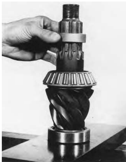
4. Remove and retain bearing spacer from pinion.
