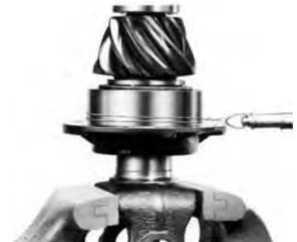
Measuring Bearing Preload with Pinion in Vise.
