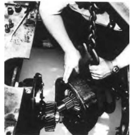
Installing Power Divider Assembly with Chain Hoist and Sling.
