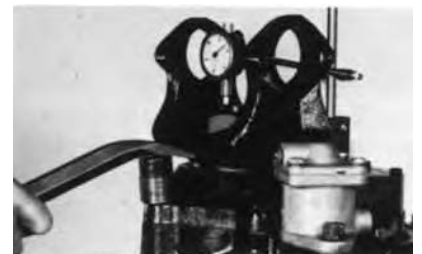
Measuring Input Shaft End Play with Dial Indicator.
