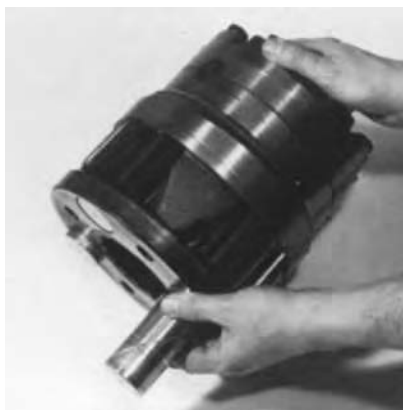
6. Invert differential assembly to remove idler pins, then remove idler pinions.
