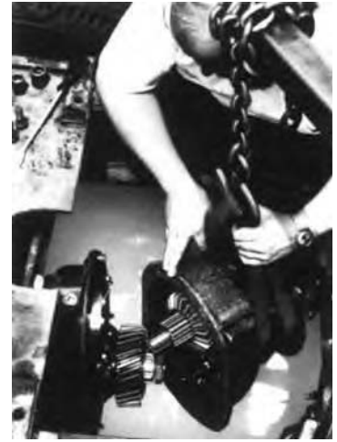
Removing Power Divider with Chain Hoist and Sling.
