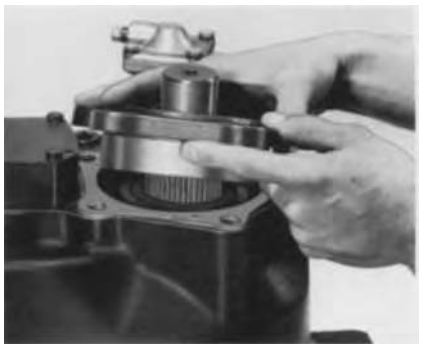
Installing Bearing Cover and Shim Pack.
