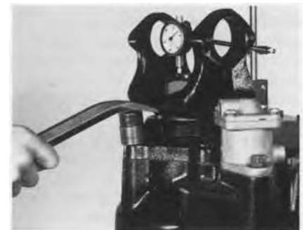
Measuring End Play with Dial Indicator.
