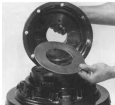
2. Remove small support case and thrust washer.
